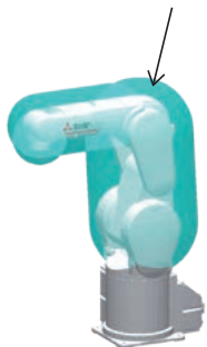
Monitoring points: 4 locations on the robot arm
